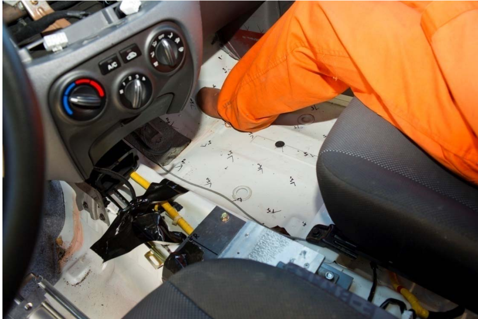
Figure 3-31 – Floor Board of test vehicle after Test 110MASH2C14-01
