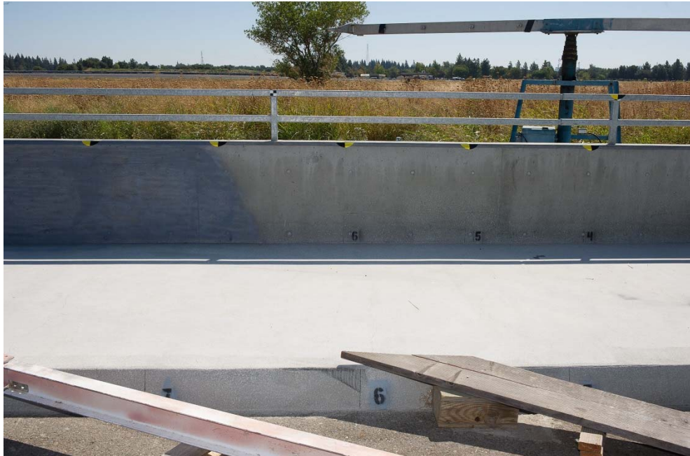
Figure 3-12 – Type 732SW test article prior to 130MASH3C13-02
