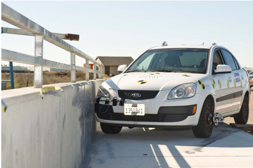
Figure 3-28 – Test vehicle prior to impact for Test 110MASH2C14-01
